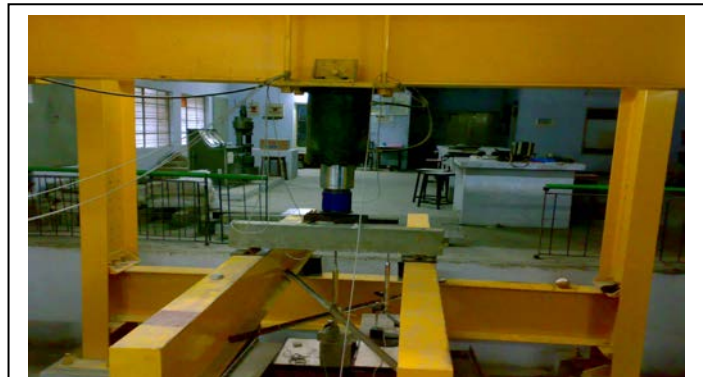
Figure 2: Photo showing 100 ton loading frame - Arrangement of test specimen
